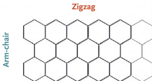
Fig. 4: 0 degree (armchair) or 30 degree (zigzag) fold edges.
