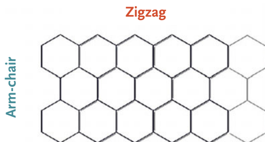
Fig. 4: 0 degree (armchair) or 30 degree (zigzag) fold edges.
