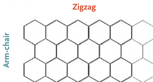
Fig. 4: 0 degree (armchair) or 30 degree (zigzag) fold edges.
