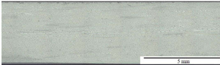
Fig. 9: Micrograph of sample cross-section, showing more fibers in the upper half of the thickness, marking the side of the base material.
