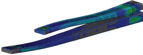
Fig. 6: FEM analysis of the GFRP-X axle
