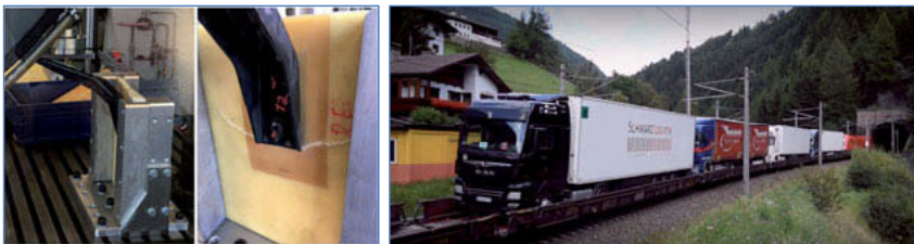
Fig. 17: Testing the connection of the aeropackage (new and aged); railroad reverse loading
