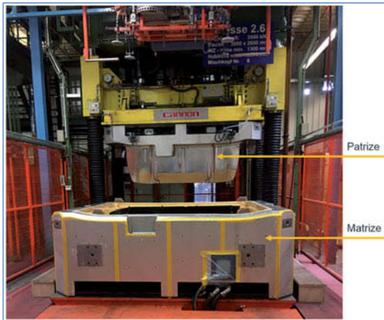
Fig. 10: RTM tool with 100% nickel surface
