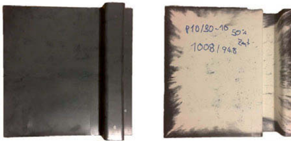
Fig. 3: Photographs of the two sides of the trial parts molded with 50% mold coverage and central charge placement.
