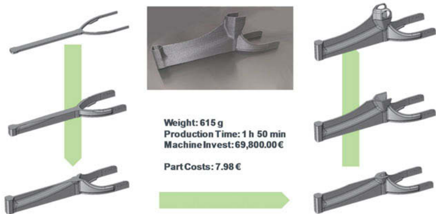
Fig. 6: Topology-optimized design for pellet extrusion additive-manufacturing processes
