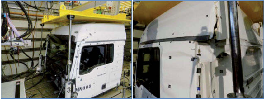
Fig. 14: First component test with anchored body
