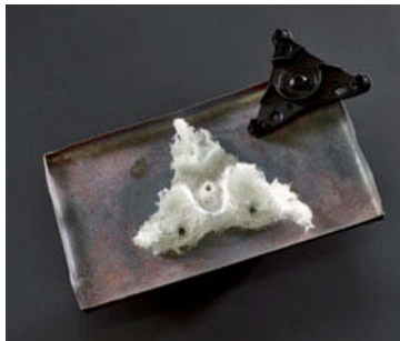
Fig. 5: Housing (right) and fiber content after ashing (middle) (source: ARBURG GmbH + Co KG)
