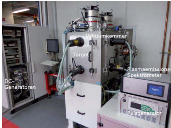
Fig. 3: HiPIMS system at the Kunststoff-Institut Lüdenscheid equipped with a Magpul MP 2 pulse generator and a Plasus Emicon plasma emission spectrometer (source: Kunststoff-Institut Lüdenscheid GmbH)
