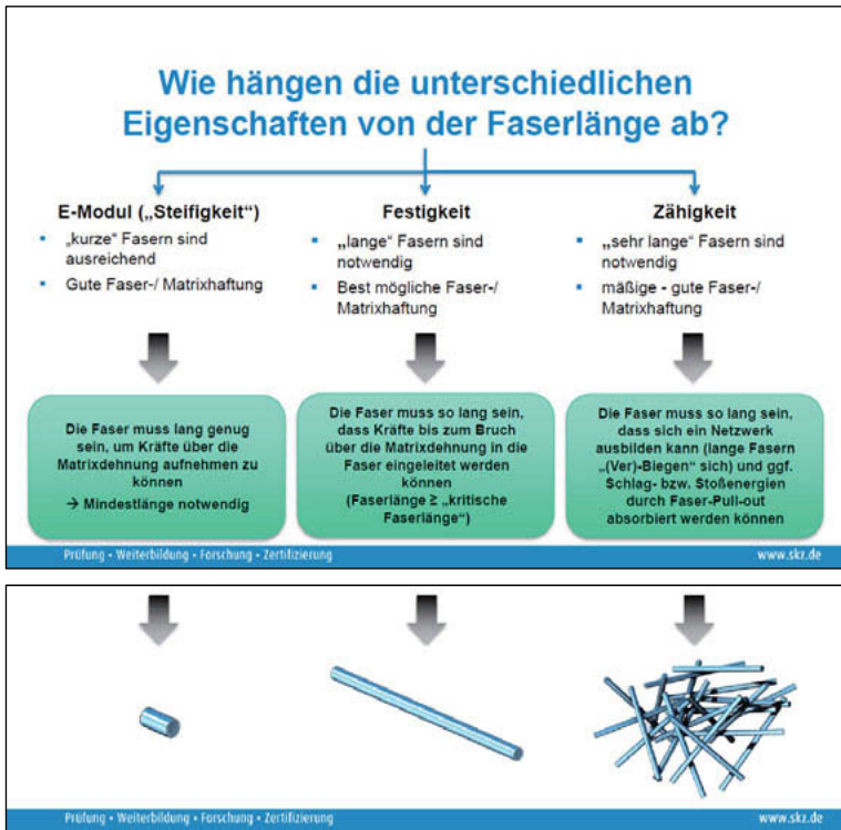
Fig. 1: Dependence of the component mechanical properties on fiber length (source: SKZ)
