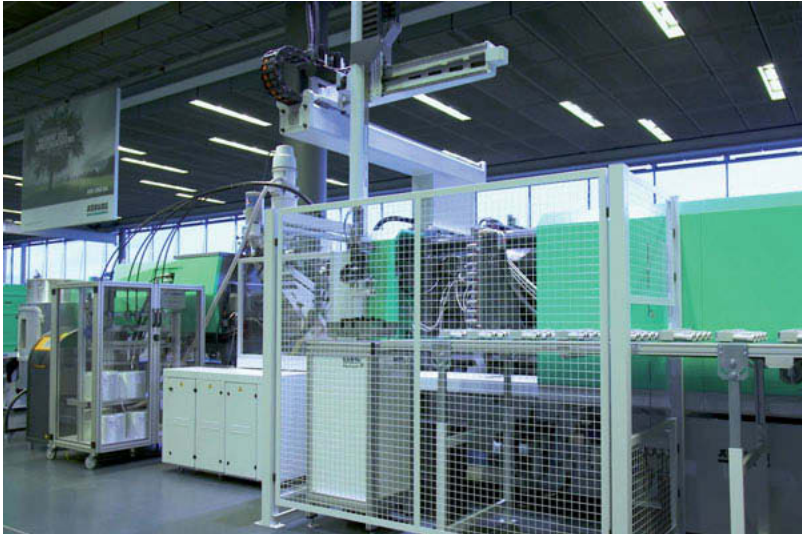
Fig. 6: Production cell with FDC unit as well as automated handling and weighing of the fiber-reinforced components (source: ARBURG GmbH + Co KG)
