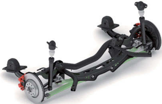
Fig. 7: Assembly of the GFRP-X axle [1]
