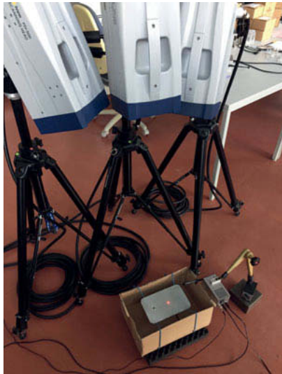
Fig. 7: Test setup with PSV-500-3D and SAM.
