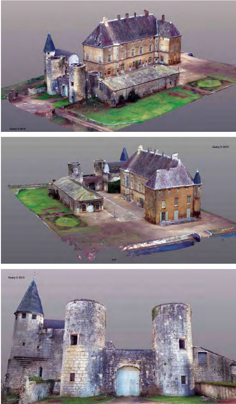
Figure 19.3. Photogrammetric survey of architecture, the Château de Germolles (see chapter 4). © Julien Guery, 2015.
