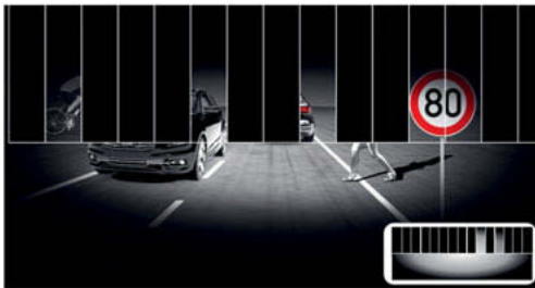
Fig. 2: Situation illuminated with fixed low beam and adaptive driving beam by addressable LEDs
