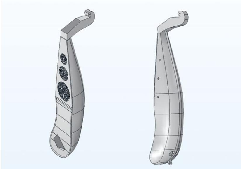
Fig. 1 The three-dimensional computer model of a Moroccan *rabāb* used for simulation. For the vibrational analysis the strings and tuners are not included, as only the vibrational characteristics of the instrument body are of interest. String tension is still taken into account.
