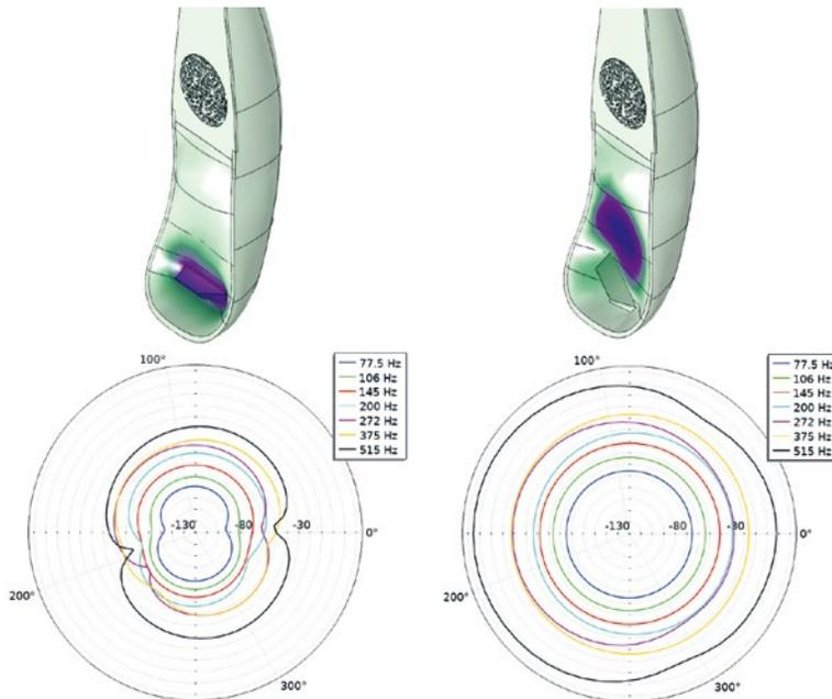
Fig. 2 Top: exaggerated displacement of the *rabāb* membrane when the bridge is excited at 250 Hz in the case of a perpendicular and an angled bridge. Bottom: Radiation characteristics calculated for both bridge settings.
