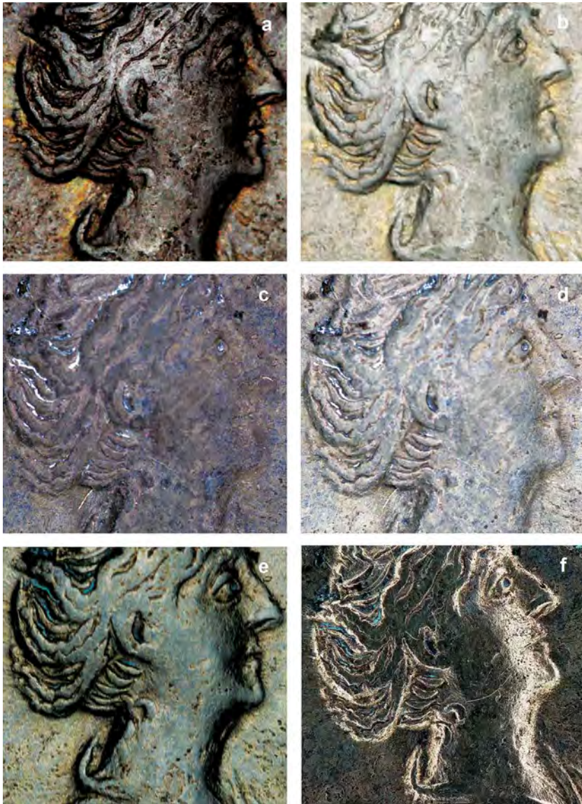
Figure 3.5. Appearance of coin A obverse, detail: (a) RTI from dome 1; (b) RTI from dome 2; (c) RTI from dome 3, albedo mode; (d) RTI from dome 3, ambient mode; (e) RTI from dome 4; (f) focus stacked picture.
