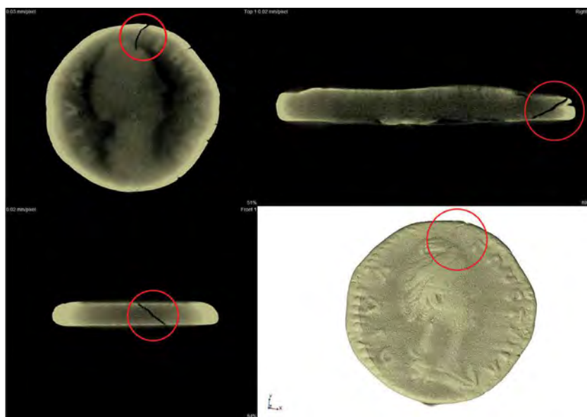
Figure 3.11. Crack inside coin B visualized by microCT method (three perpendicular microCT sections and rendered 3D model). © Miroslav Hain, 2014.
