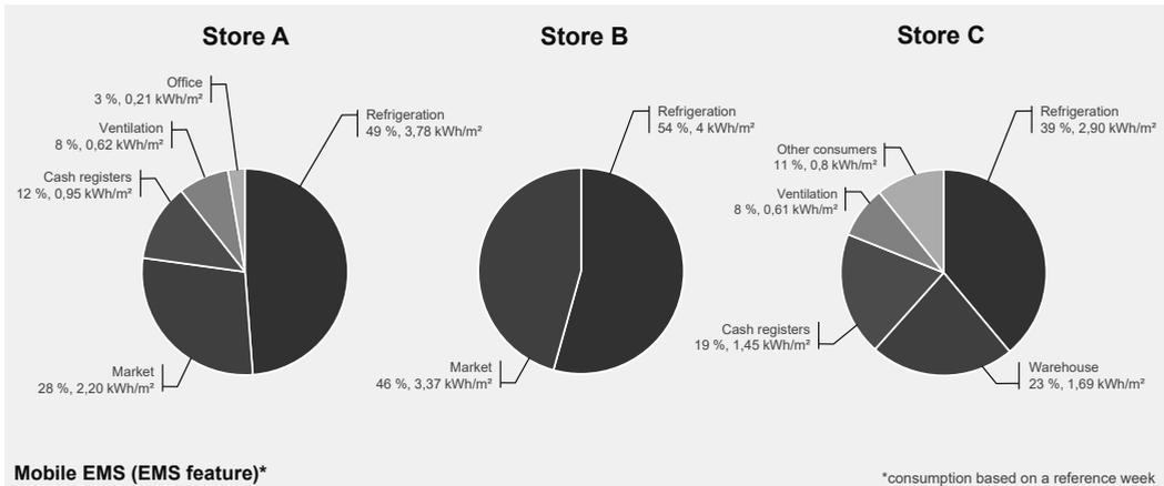
Figure 4: Consumption disaggregation and consumer-specific EnPIs per m<sup>2</sup> sales area based on the mobile EMS
