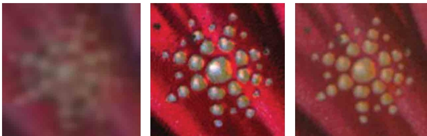
Figure 8.7. Russian icon detail extracted from the different devices to show the spatial resolution quality from three IS systems.
