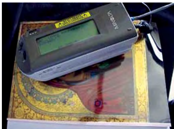
Figure 8.3. Minolta CM-26000 measuring reflectance spectra on selected areas of the Russian icon.
