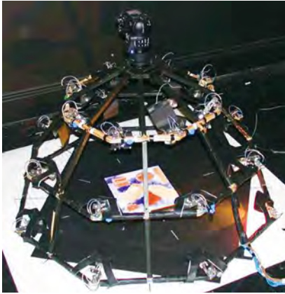
Figure 20.1. Left: experimental apparatus for PTM at the National Gallery (London) with twenty-four tungsten spotlights mounted on a rigid framework. Below: surface relief of a painted test panel, lit from the top right. © Joseph Padfield, National Gallery, London.
