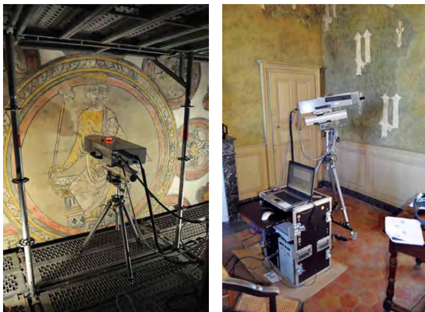
Figure 17.1. LIBS in operation at Chartres Cathedral (left) and Château de Germolles in Burgundy (right). © LRMH, 2011 and 2015.
