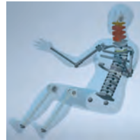
Fig. 3: Validation device 50-percentile female rear impact seat evaluation tool VIVA II (Source: http://crashscene.se/f50flogard )
