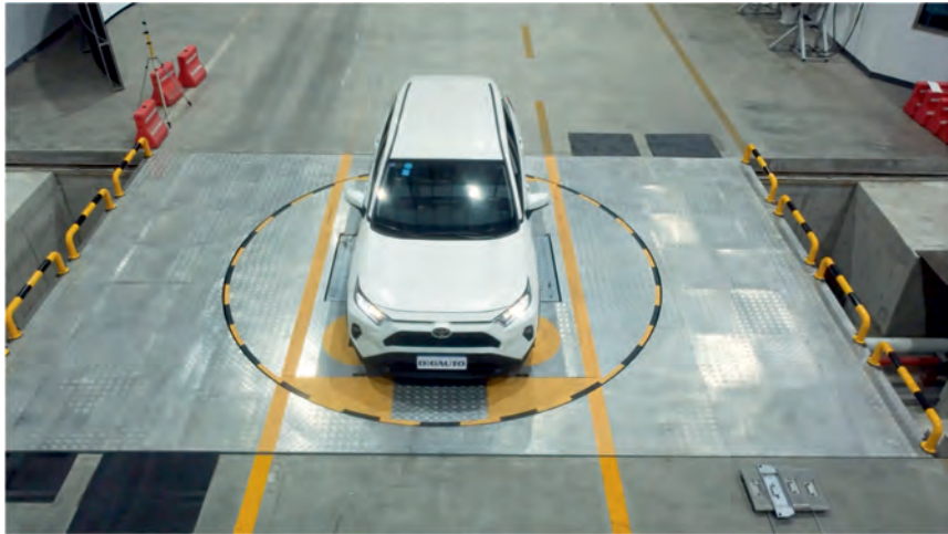
Fig. 3: The rotating and transversally moving Platform of VTEHIL.
