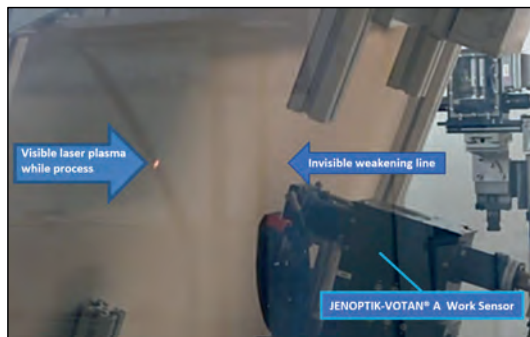
Picture 07: Laser Airbag Weakening: Roof trim processing
