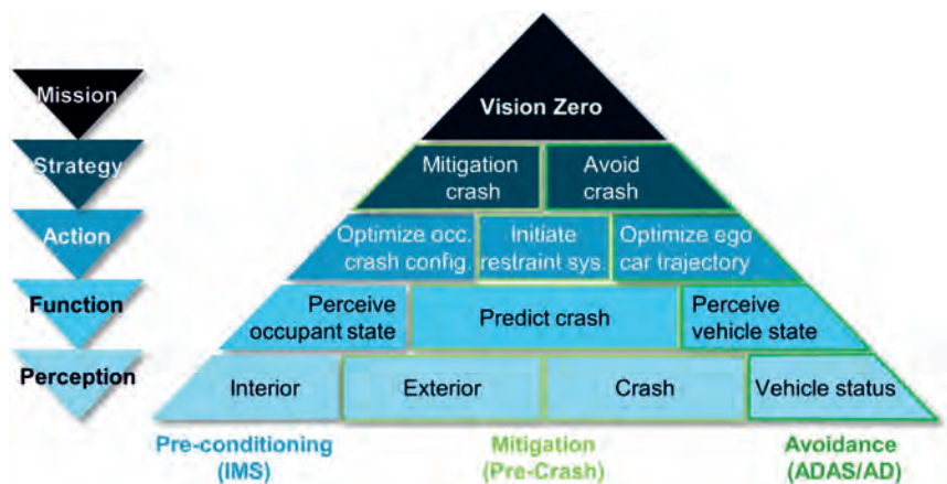
Fig. 1: Predictive Safety Pyramid – Holistic Top-Down Safety Systems Engineering based on enhanced perception techniques (IMS: Interior Monitoring System).
