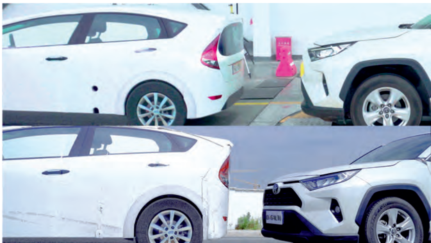
Fig. 4: Comparison of Test with GVT on VTEHIL (upper) and Proving Ground (lower)
