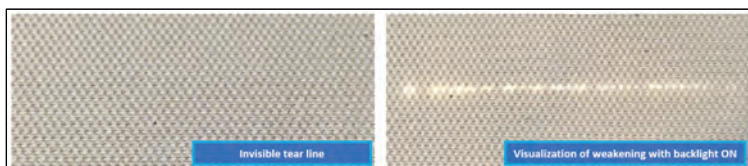
Picture 08: Laser Airbag Weakening: Roof trim processing result
