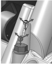
Fig. 19: Modular valve train system overview – focus on the oil relief holes
