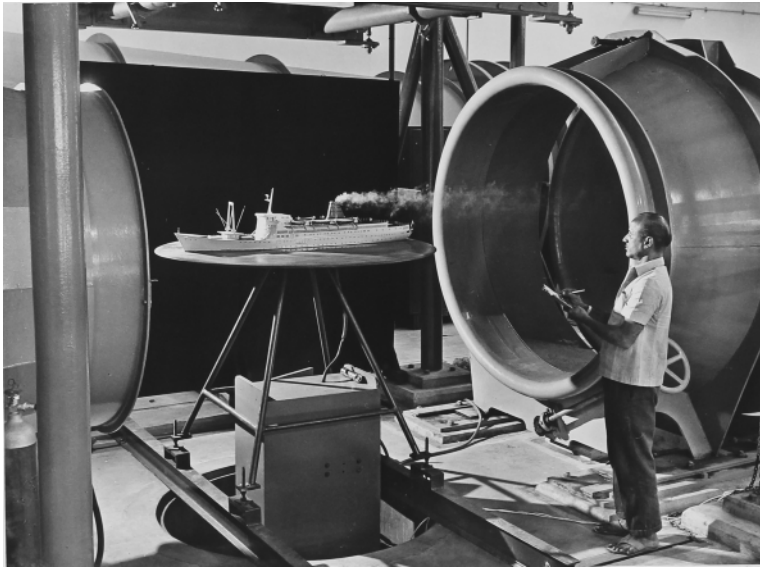
Fig. 2: A model of the SS State of Bombay, built by M/S Mazagon Dock Ltd., in the 1.5-m-diameter test section of the closed-circuit, low-speed wind tunnel at the Department of Applied Mechanics, IIT Madras. This wind tunnel was capable of a maximum speed of 60 m/s and was provided with a semi-automatic six-component balance. Photographed by Cadambi Gourishankar (Photo: Heritage Centre, IIT Madras).
