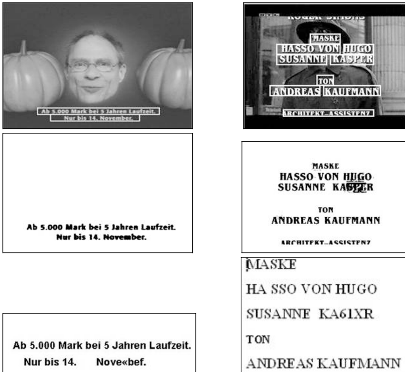
Figure 3: The images on the top row show the result of text localization. The middle row depicts the results of the text segmentation process, in which the background has been removed and the text has been marked black. In the last row, the result of the recognition software (OCR) is shown.
