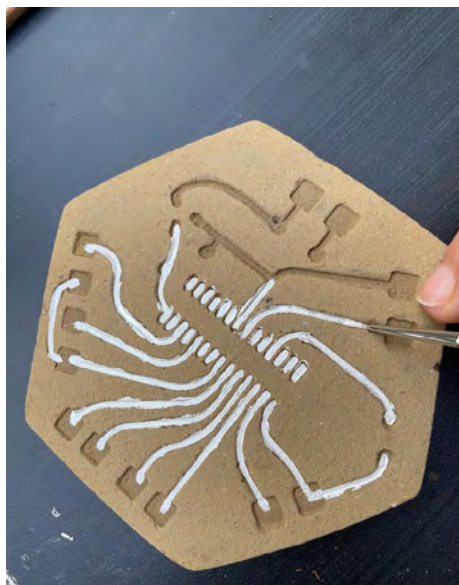
Painting the PCB circuit on the clay boards with silver ink, Burgenland, Austria, October 2023 © Patrícia J. Reis
