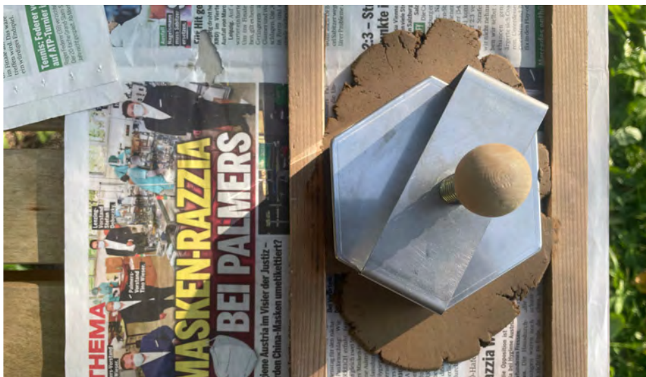
Cutting the hexagon shape using a tile cutter, Burgenland, Austria, October 2023 © Patrícia J. Reis
