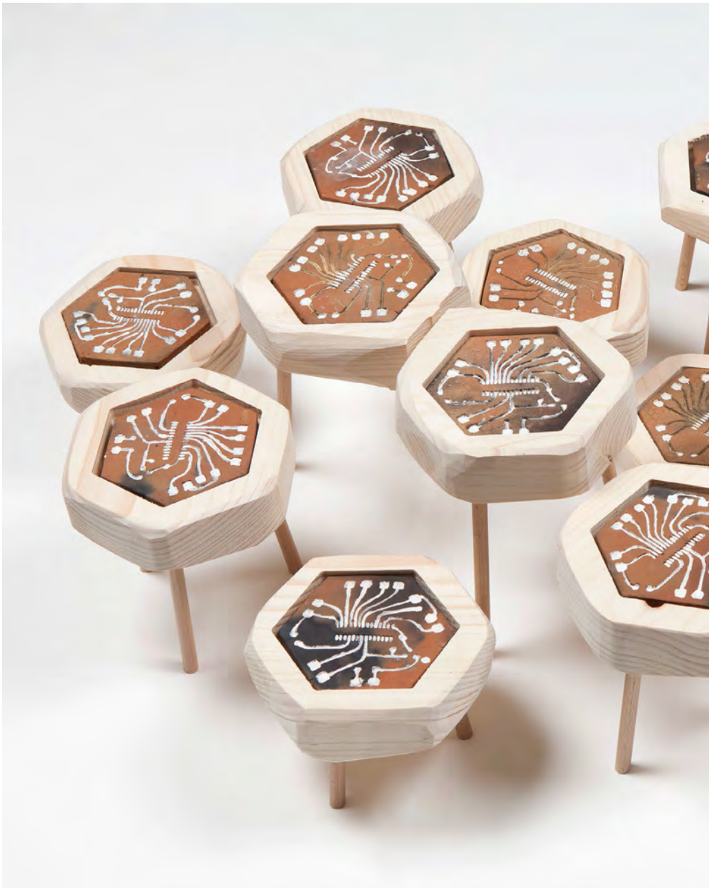
Boards after being fired, before soldering the electronic components © Janine Schranz
