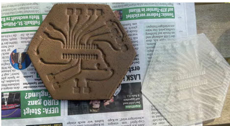
'Stamping' the circuit into the clay with the 3D-printed 'stamp', Burgenland, Austria, October 2023 © Patrícia J. Reis
