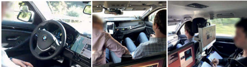
Fig. 1: Bosch Wizard-of-Oz vehicle: Environment for test participant (left); wizard driver on the co-driver seat (middle); experimenter and HMI wizard on the back seat (right).
