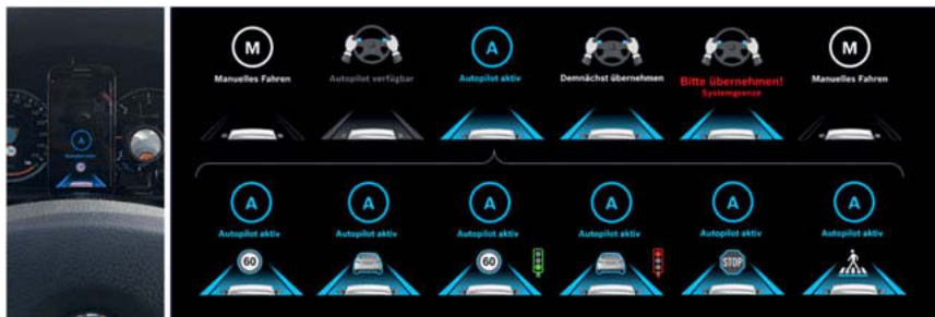
Fig. 2: Visual HMI showing basic system states (top row) and additional system information while in L4 automated mode (bottom row). The graphics were displayed on a smartphone device installed in front of the instrument cluster.
