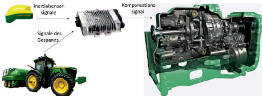
Fig. 4: System architecture and components of the smart power train control
