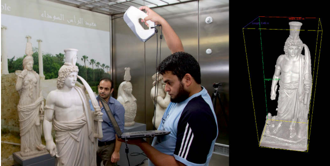
Fig. 1: (Left) Mohammed Elfarargy from the BA ICT Sector scanning one of the temporary artefacts of the BAAM collection using the Artec Eva handheld scanner; (right) the final 3D model.
