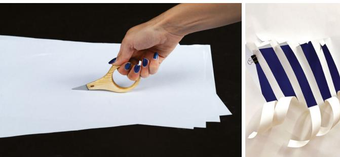
*'The ring' final prototype out of timber and metal, being tested by Nadja, was used as a standard cutter.*
