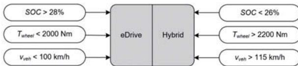
Fig. 3: Rule-based control strategy for driving mode selection
