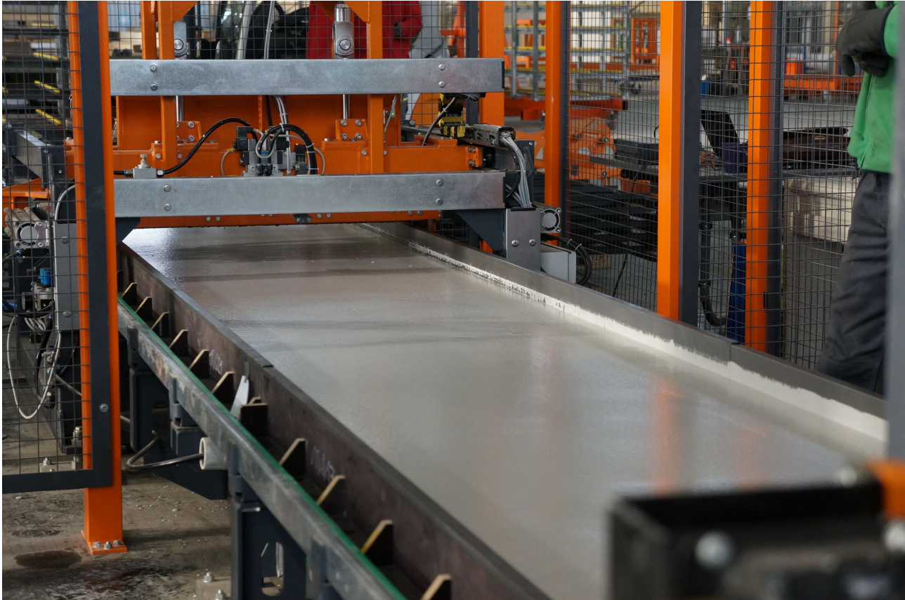
Abb. 16: Co-Extrusions-Technologie, Aeroleichtbeton © G.tecz Engineering GmbH
