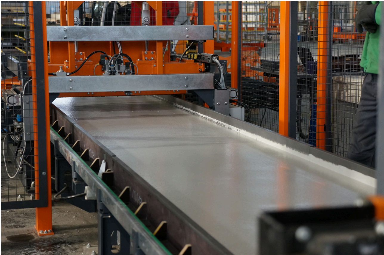
Abb. 16: Co-Extrusions-Technologie, Aeroleichtbeton © G.tecz Engineering GmbH
