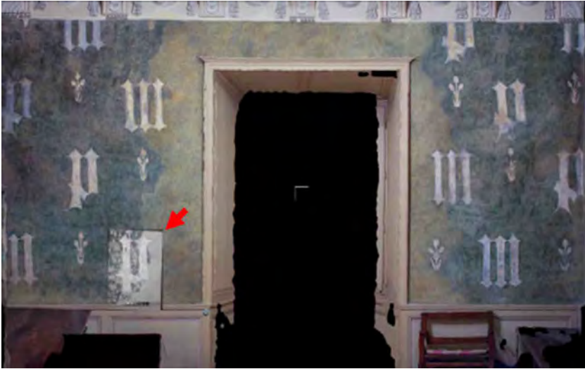
Figure 4.15. Snapshot from the SIVT application tested on Germolles case study data. The rectified and registered IR image of the P (red arrow) is displayed on top of the orthophotography of room dn south wall. Photos: Stefanie Wefers and Tobias Reich, 2016 and Francesca Piqué, 2013.
