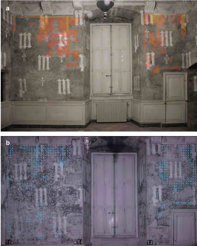
Figure 4.13. (a) Graphical representation through IRT of areas of detachment in the north wall of room dn; (b) representation (overlaid onto an IR image) of similar areas, in blue, as recorded by tactile assessment (knocking method). Photos: (a) Cristina Tedeschi and Marco Cucchi; (b) Nutsa Papiashvili, 2015.
