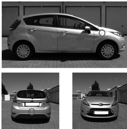
Fig. 1: Mounting positions of KESS sensor for damage detection inside the vehicle body
