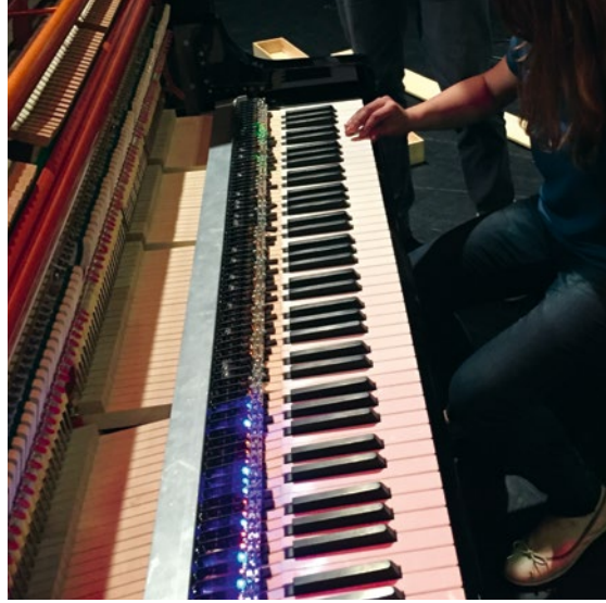
Fig. 1 The first of two prototypes of the hybrid piano (with magnetic sensors). Hardware created by the engineer Darko Lazović.
