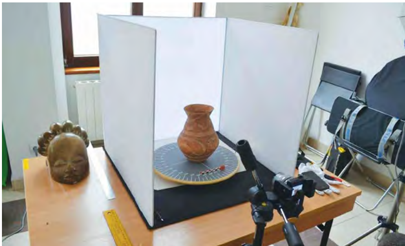
Figure 6.2. Setup for photogrammetric acquisition of the ceramic vases. © National Museum of Romanian History, Bucharest, 2015.
