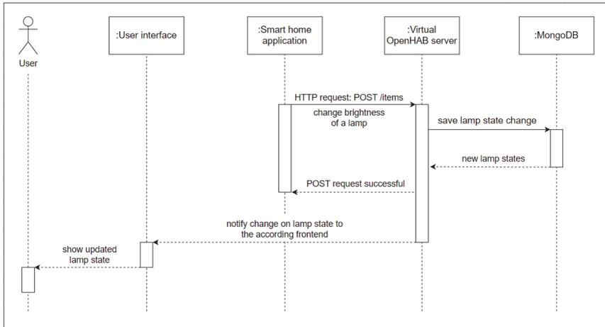
Figure 3. Sequence diagram of a typical scenario
