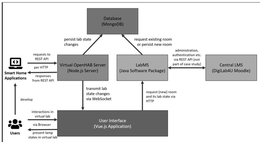
Figure 1. Architecture and components of the application
