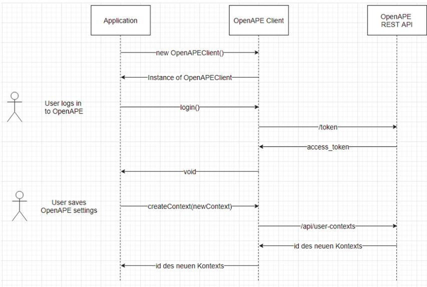
Figure 2: Sequence diagram for an example workflow
