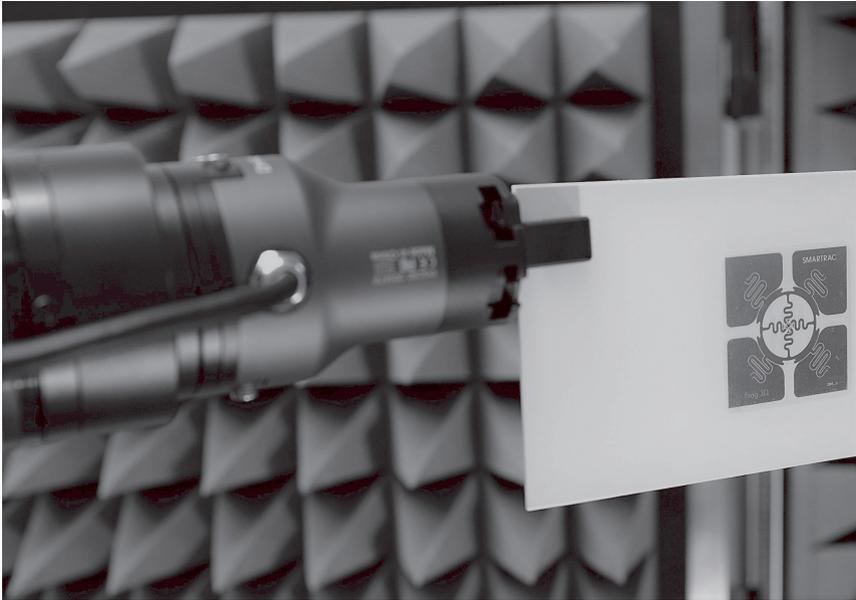
*Figure 2: A UHF RFID-transponder ready for testing—a visual inspection shows information about the manufacturer (Smartrac) and the antenna design (Frog 3D). The square layout indicates orientation insensitivity to horizontal or vertical usage.*
