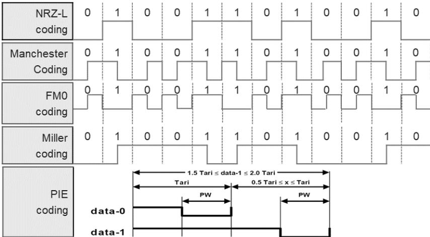
Figure 8: Methods of coding (Source: Rizzi et al., 2011)
