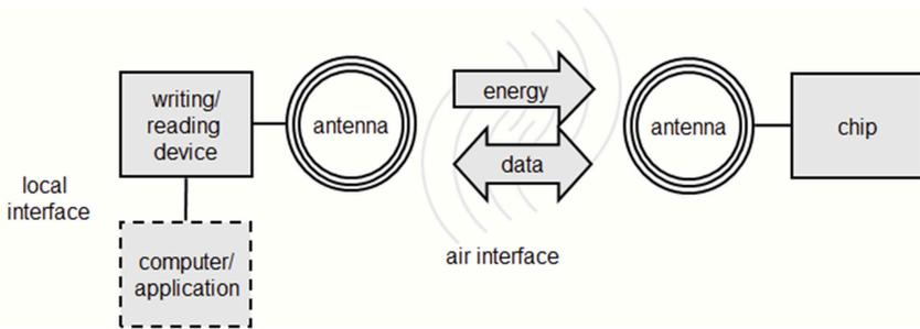
Figure 2: Components of an RFID System (Finkenzeller, 2010)
