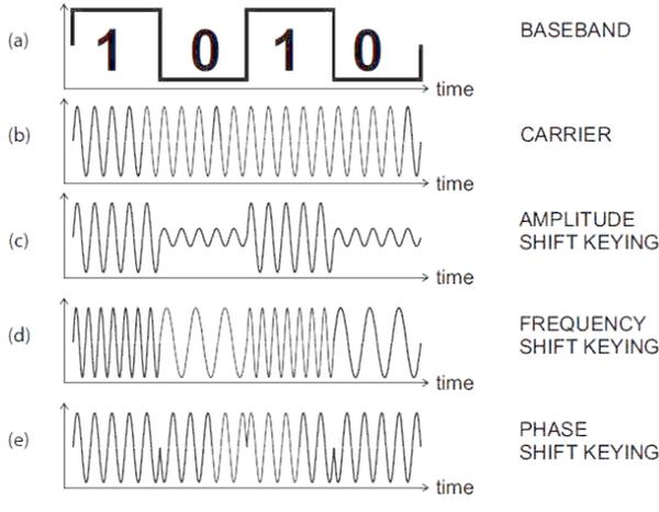
Figure 7: Methods of modulation (Kaur & Kaur, 2015)
