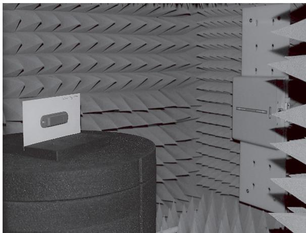
Figure 6: The RFID measurement cabinet inside, turntable with a blue RFID-transponder on a white plastic substrate to the left; linear polarized reader-antenna on the right; surrounding absorbers
