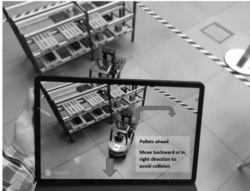
Figure 8 AR supported interaction and feedback GUI
