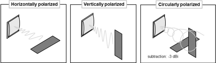
Figure 6: Antenna polarization
