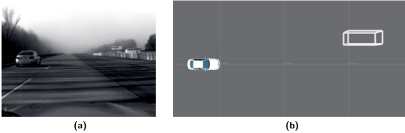
Figure D.2: A scene from an overtaking maneuver scenario used for evaluation, as seen from a camera sensor (a) and the 3D visualization software (b), where the ground truth for the target vehicle is represented as a white wire-frame box.
