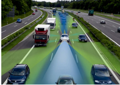
Figure 1.19: Surround environment perception for automated driving on highways using laser scanner (green), radar (blue), camera (white) and ultrasonic (dark green) sensors.
