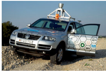
Figure 1.17: MuCAR-3: Research vehicle for autonomous driving in off-road environments from the Universität der Bundeswehr in Munich, Germany (Image Source: [297]).
