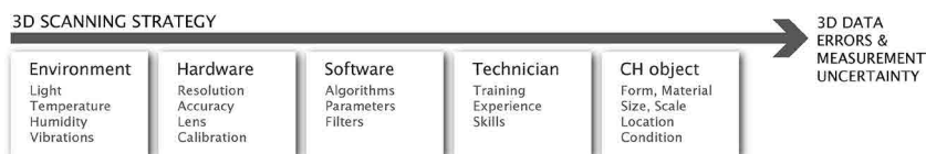
Figure 1.1. Example of sources of measurement error in 3D scanning that lead to uncertainty of measurement results (Moitinho de Almeida 2013).
