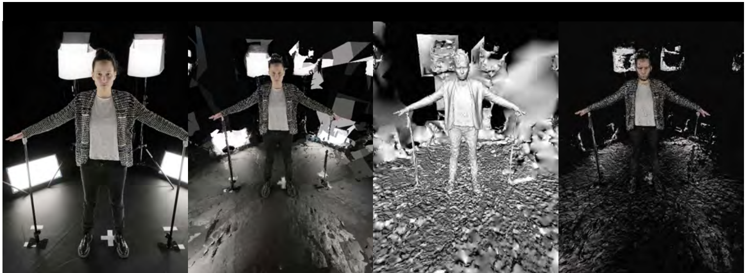
FIG. 1 PHOTGRAMMETRY PROCESS WITH THE SOFTWARE REALITY CAPTURE . ORIGINAL PHOTO, POINT CLOUD RECONSTRUCTION, 3D RECONSTRUCTION WITHOUT TEXTURE, 3D RECONSTRUCTION WITH TEXTURE.
