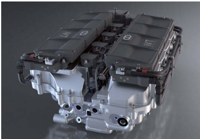
Fig. 12: 16 valve, 4 cylinder in-line iVT package – based on the Jaguar Land Rover Ingenium engine
