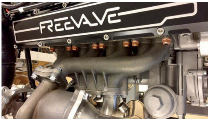
Fig. 1: Divided Exhaust Period manifold
