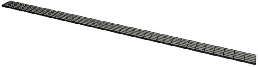
Figure 6.66: Computational mesh used for the discretization of the electric, thermal, and structural field of the bimetallic beam.
