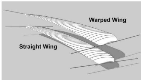
Figure 2: Illustration of Wright concept of “wing warping”<sup>113</sup>
