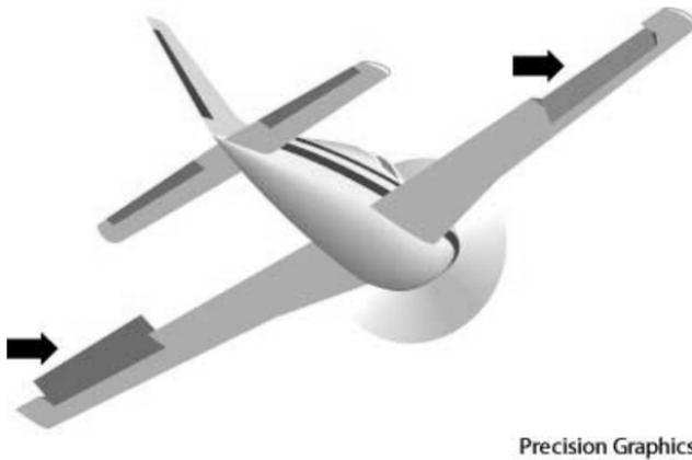
Figure 3: Ailerons (moveable) with fixed straight wing of modern aircraft<sup>114</sup>
