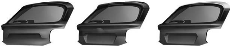
Fig. 7: One “tailgate backbone” for different vehicle designs
