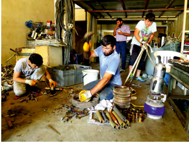
Figure 5.11: Dismantling elevator parts 15
