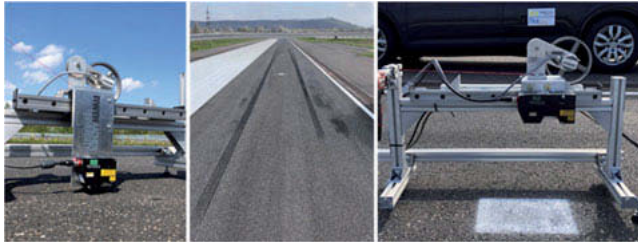
Fig. 3: Microtexture (left) and macrotexture (right) 2D/3D profilometer for surface topography characterisation at the track.
