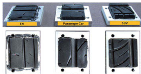
Fig. 12: Prepared tyre rubber samples 60x60 [mm 2 ] after conditioning.
