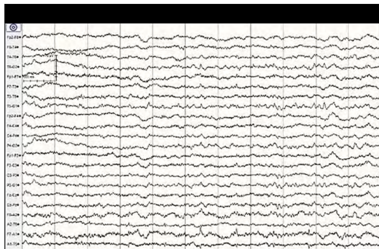
FIG. 1 EXAMPLE OF EEG SIGNALS. EACH LINE REPRESENTS THE SIGNAL MEASURED AT A SPECIFIC ELECTRODE LOCATION ON THE SCALP.
