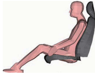
Fig. 13. Full body human model interacting with a car seat, where seat and soft tissue compliance is modelled using stress-penetration curves.
