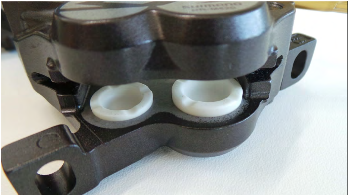
Fig. 7: Brake calliper with differing piston diameters
