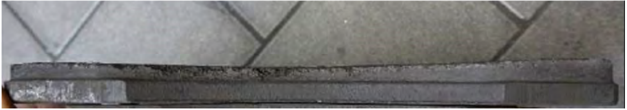
Fig. 4: Diagonal wear of a brake lining
