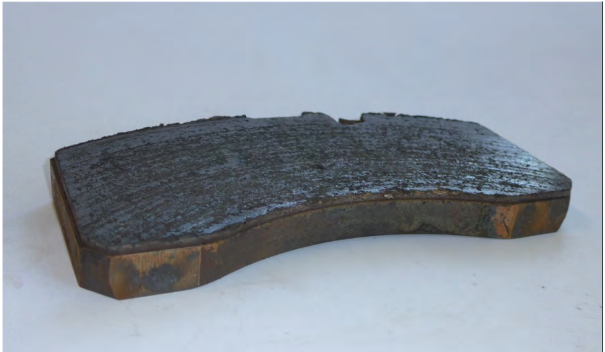
Fig. 15a: Linings after completing the driving trial
