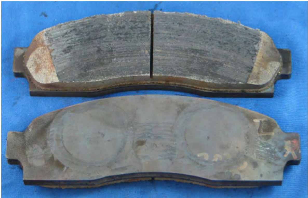
Fig. 15. NU-15D-AKM2023; phenolic-core LCB pad / chamfered, after SAE J2522 AK Mater brake performance testing.
