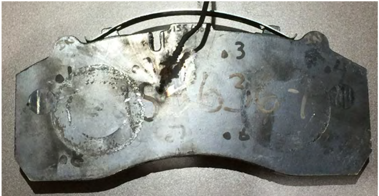
Fig. 5. Post-test D1203 pad with light-weight composite back-plate (LCB), following ISO 26865 test procedure.
