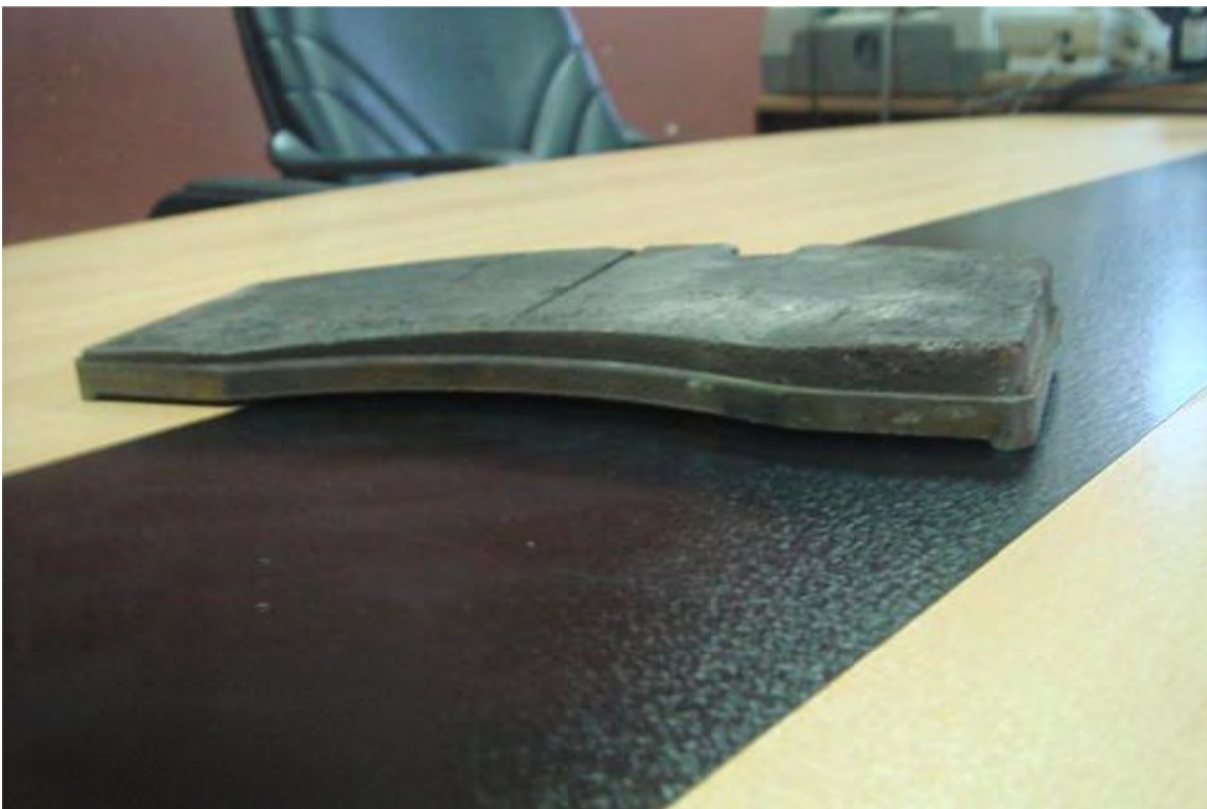
Fig. 3: Diagonal wear of a brake lining
