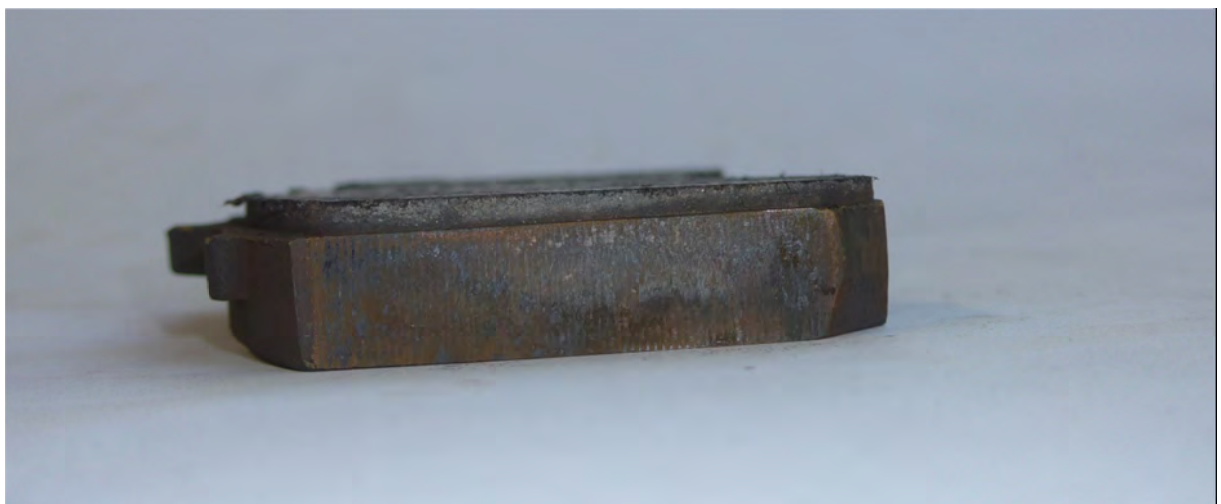
Fig. 15a: Linings after completing the driving trial
