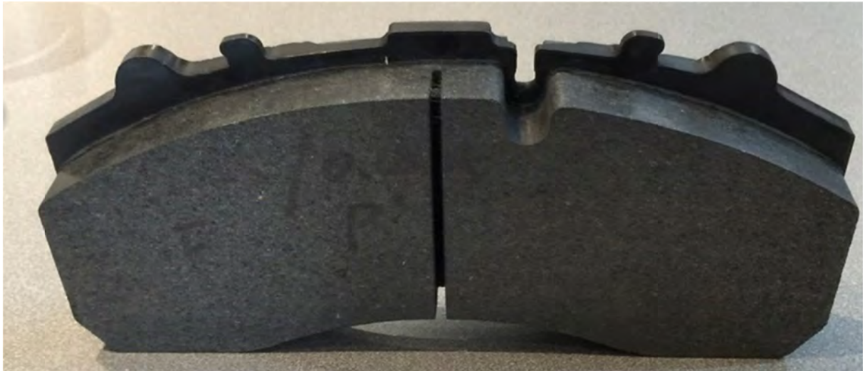
Fig. 4. Completed phenolic composite disc brake pad; FMSI Ref. D1203
