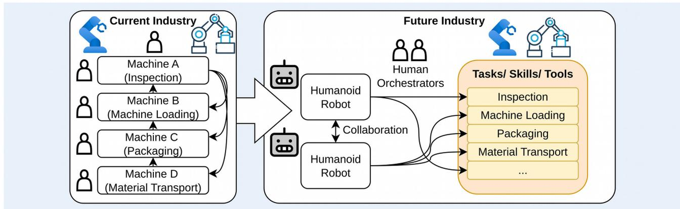
**Fig. 1** From fragmented automation to embodied integration: Paradigm shift from siloed, task-specific systems to versatile humanoid agents orchestrated by humans. *Source: Fraunhofer IPA*
