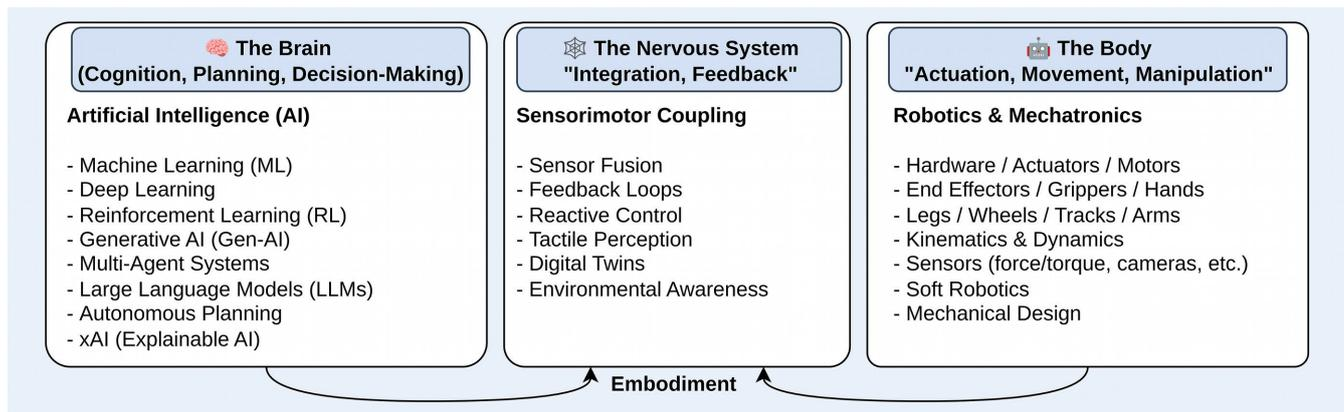
**Fig. 3** Three core components of embodied autonomy: brain (AI), body (robotics), and nervous system (sensorimotor integration) enabling intelligent, adaptive physical agents. *Source: Fraunhofer IPA*
