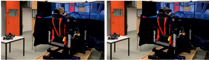
Figure 7: AUDEx – real world setup: Driving Race Pilot with triple-screen setup (left) or HMD (right)
