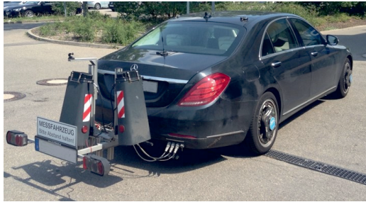
Figure 3.1: Test vehicle used for SWB measurements
