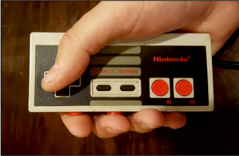
Figures 1 and 2: One-hand NES controller with buttons on the bottom; Rewired and inverted left-hander controller
