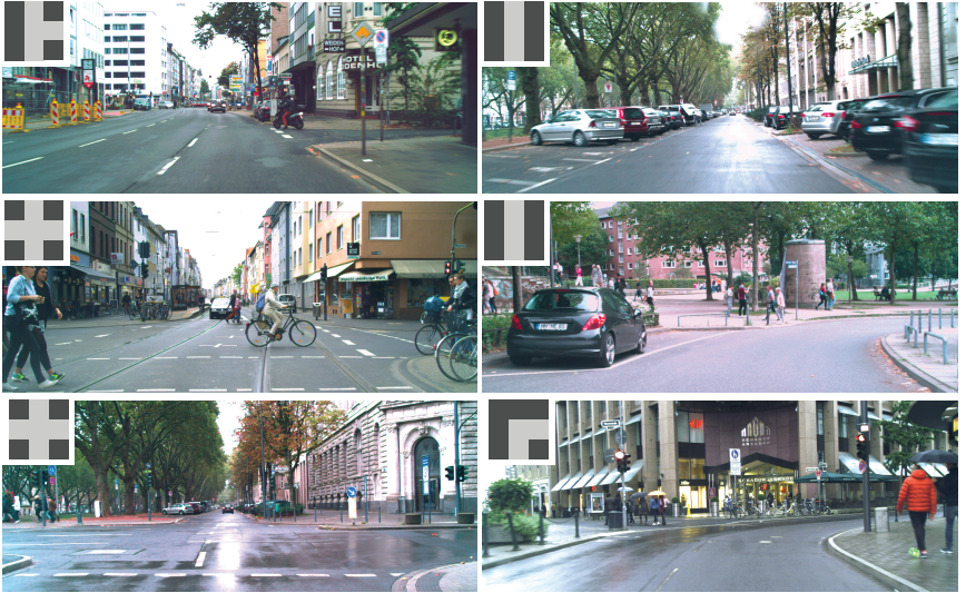
Figure 5.6: Example images from the test partition of the dataset with overlaid road topology predictions. From top left to bottom right, the corresponding ground truth classes are: junction right, straight road, intersection, turn right, intersection and turn right.
