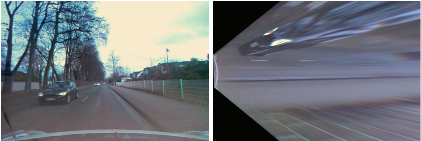
Figure 3.5: Example image of a traffic scene recorded from the test vehicle and the corresponding image after applying the BEV transformation.
