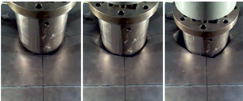
Figure 5.15: Rupture behaviour of the outer hull for Experiment 3.
