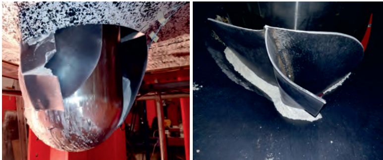
Figure 5.28: Ripped outer hull after indentation of the inner hull (left). The remaining flap in the inside of the box can be seen in the right image.
