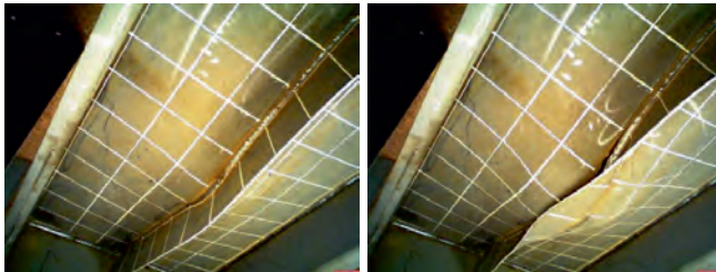
Figure 5.22: Deformation of a single stiffener as can be seen in [29] (from [29]).
