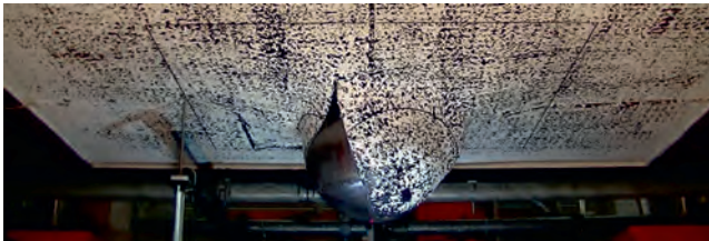
Figure 5.6: Flap occurring at the inner hull after rupture in the first experiment.
