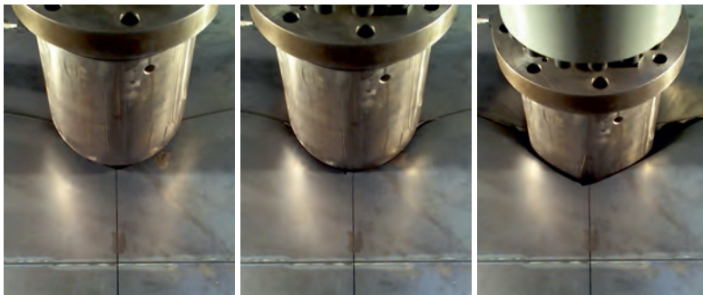
Figure 5.24: Rupture of the outer hull for Experiment 5.
