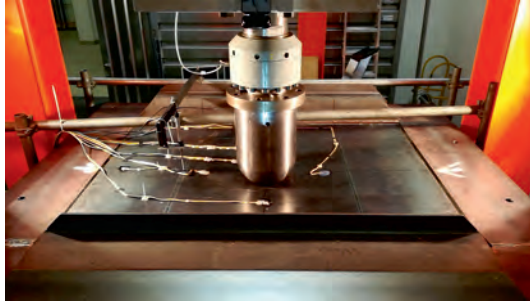
Figure 5.3: View on the experiment at the beginning of the penetration of the outer hull. Deformations and stresses are measured for comparison.
