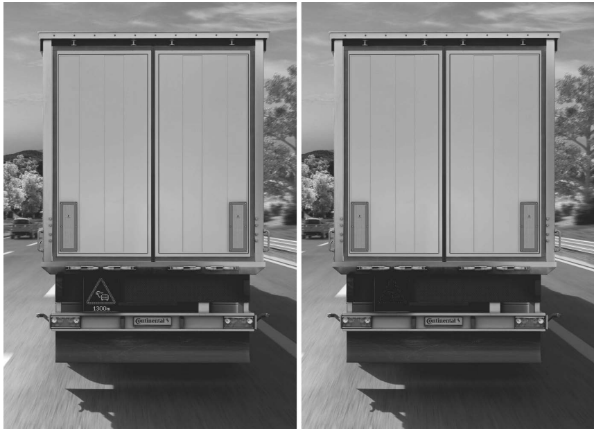
Fig. 13: Possible marking of the truck to inform the subsequent traffic. Right: during normal driving. Left: warning during eco coasting. Additionally, the sign could be set into a blinking mode in order to draw more attention to the sign.
