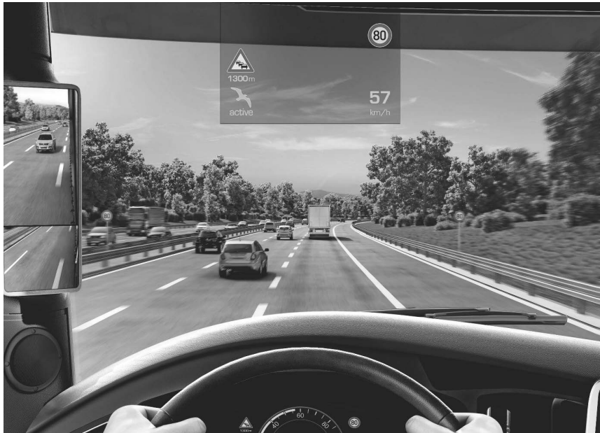
Fig. 12: Desirable HMI information for the driver during predictive eco coasting events. Here: via head up display information on the windscreen via head-up display.
