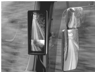
Fig. 3: Comparison of a digital mirror system with the view of a conventional truck mirror
