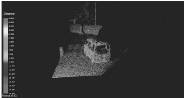
Fig. 7: Result of a Flash-Lidar measurement. Intensity of the reflected laser light is shown. By color coding also the distance measurement is given very accurately.
