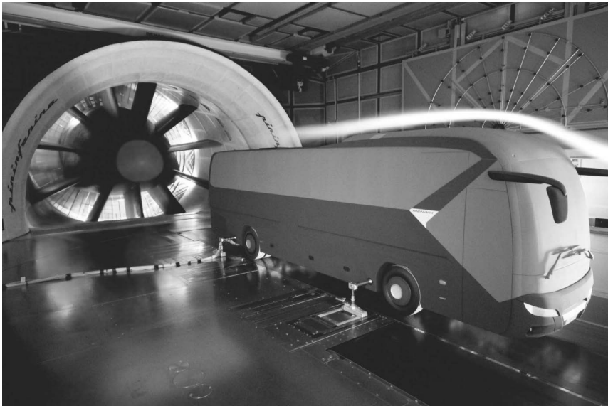
Fig. 5: The aerodynamic and flow-optimised exterior of the NEOPLAN Tourliner
