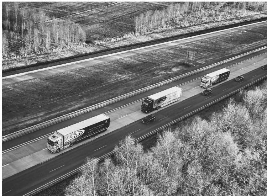
Fig. 2: Platooning with Highway Pilot Connect (© Daimler AG)
