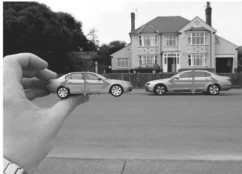
Fig. 6: Optical picture of two cars. With a mono camera and object detection it is difficult to correctly detect the scenario. With the additional time of flight measurement of a Li-dar-sensor the scenario is clearly recognized.
