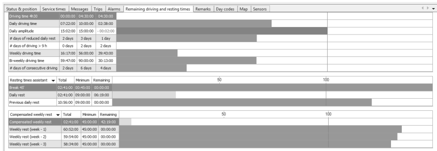
Fig. 3: Cockpit view for the real-time remaining driving and resting times for 1 driver in Transics telematics portal
