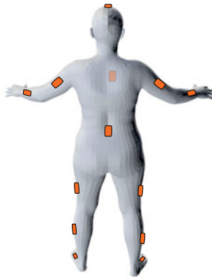
Figure 2.9: IMU placement of TotalCapture dataset. IMUs are located at feet, shanks, thighs, lower arms, upper arms, sternum, waist and head.
