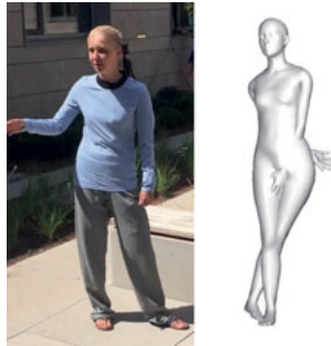
Figure 4.2: Illustration of IMU heading drift. The sensor heading errors have accumulated after a longer recording session and the obtained 3D pose is completely off.
