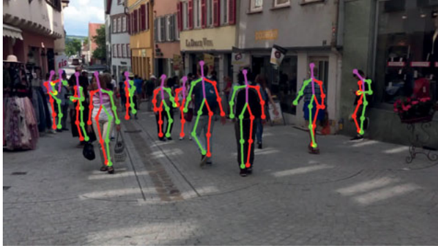
Figure 4.3: Illustration of association challenges in crowded environments. In order to combine IMU data and visual information from the camera view, 2D poses have to be associated to persons wearing IMUs. This is difficult when several people are in the scene.
