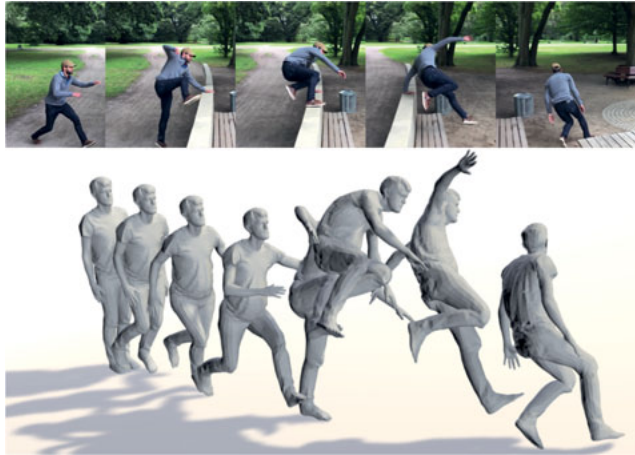
Figure 3.1: Illustration of the tracking performance using only 6 IMUs attached wrists, lower legs, back and head. The animation in the bottom row shows the output of the proposed method for a jumping sequence. The images in the top row are only shown for reference and are not part of the method.
