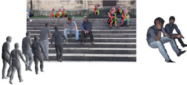
Figure 4.1: The Video Inertial Poser (VIP) combines video obtained from a hand-held smartphone camera with data coming from body-worn IMUs. It enables to capture motions of multiple people in natural environments.
