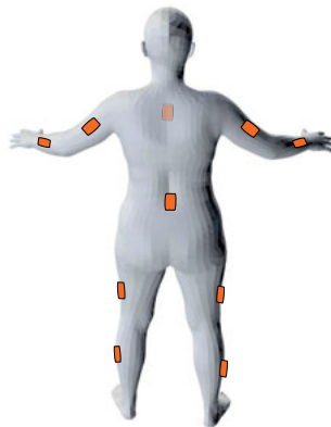
Figure 2.8: IMU placement of TNT15 dataset. IMUs are located at shanks, thighs, lower arms, upper arms, sternum and waist.
