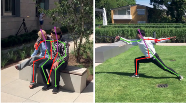
Figure 4.4: Illustrations of inaccurate 2D pose detections. Left image: current methods have trouble to correctly assign joints to persons if they are in close interaction. Right image: left and right body limbs are frequently mistaken, especially in uncommon poses.
