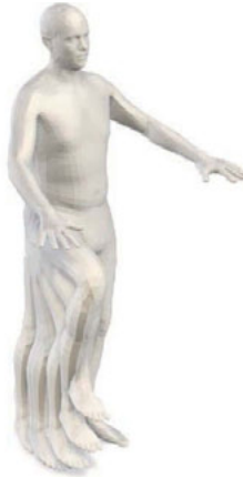
Figure 3.2: Sparse IMU orientations give only weak constraints on the full pose. Multiple knee and hip joint configurations fit well the IMU orientation of the lower left leg.
