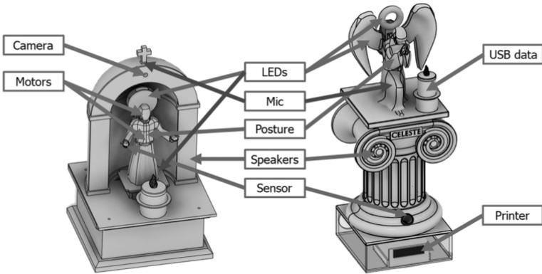
Figure 3. Components of SanTO and CelesTE: a diagram highlighting both the parts they have in common and their differences.
